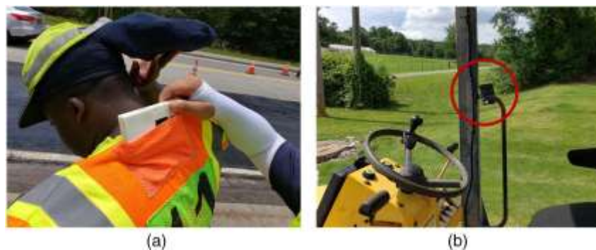
Fig. 9. (a) Placing a PPU to a worker's safety vest; and (b) EPU mounted on the equipment.
