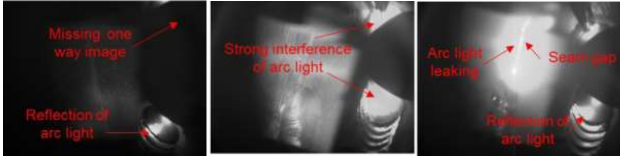
Fig. 6 Images associated with different penetration state [13]. From left to right: incomplete, complete and over penetration.
