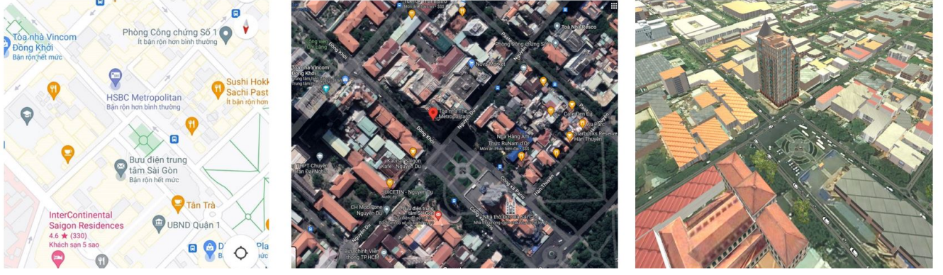
Figure 4: The modeling stage in our simulator. From left to right: (left) the 2D layout of the city map, (middle) the overlaid terrain onto the 2D city map, (right) our built 3D models such as buildings, roads, and landmark points for the city planning simulator.
