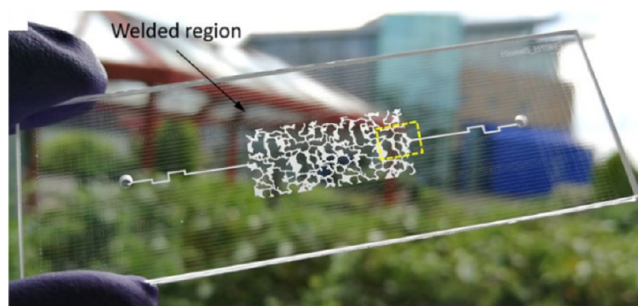
Figure 12. Glass model by laser engraving. Reproduced with permission from ref 27. Copyright 2019 Springer Nature.
