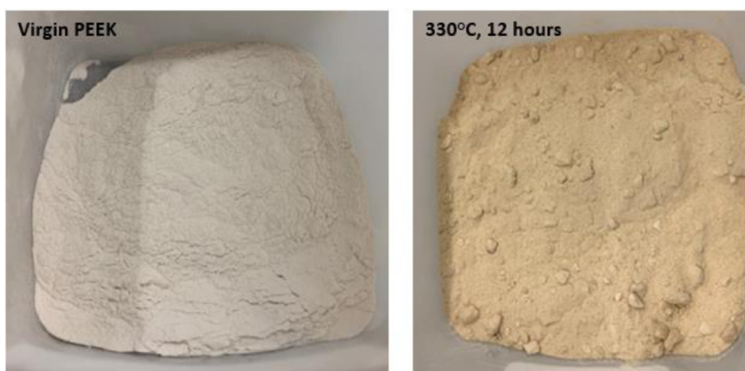
Fig. 2. Unannealed (left); 12hours annealed PEEK powder (right).
