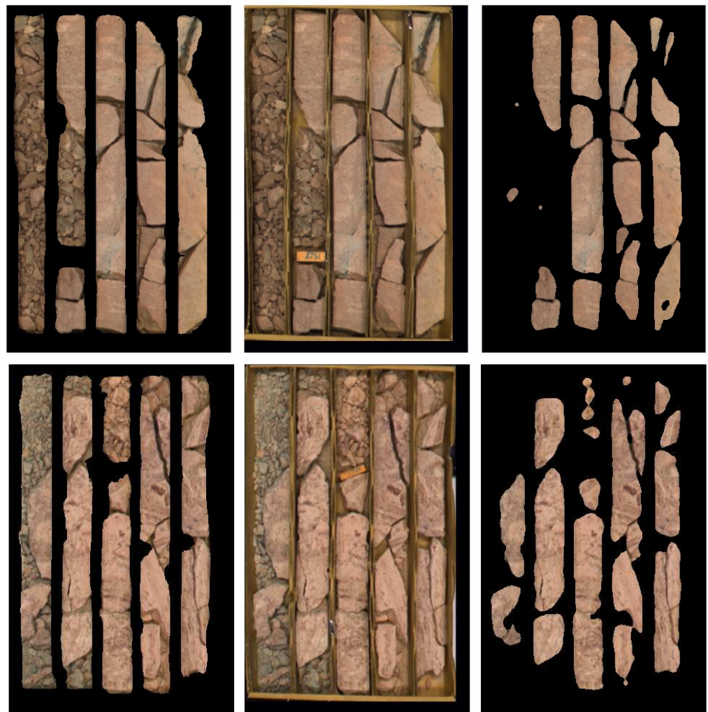
Figure 3. Masks obtained with the method described in Section 3. Each row shows a core box (middle), a neural network-generated mask (left), and a finer mask (right) that removes broken material.
