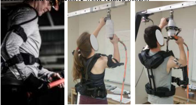
FIGURE 1: FOUR TYPES OF EXOSKELETONS: (a) power glove [22], (b) exoskeleton for arms/shoulders, (c) gravity balancing exoskeleton
