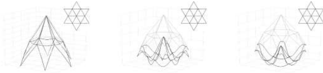
Figure 7. Primary solution branch for the hexagonal dome.
