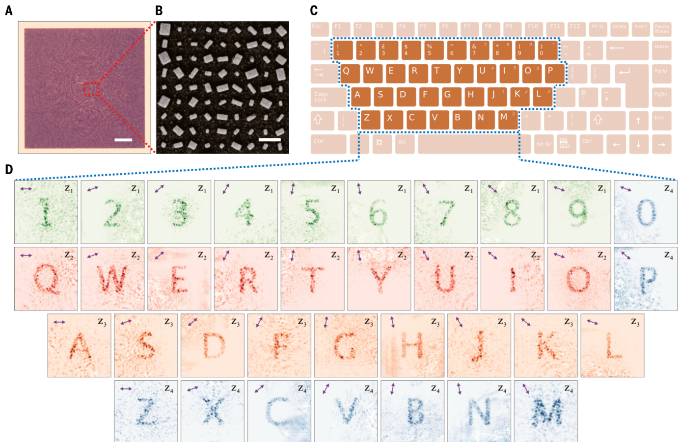
Fig. 4. Experimental demonstration of the holographic keyboard. (A) Optical and (B) SEM micrograph of the fabricated sample with simultaneously polarization- and position-multiplexed design. The scale bars are 50 \mu\text{m} and 0.4 \mu\text{m} , respectively. (C) Schematic and (D) measured results for the performance of the holographic keyboard pattern. Here we choose nine different polarization
