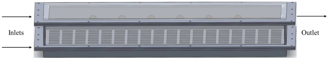
Fig. 1 A schematic of the experimental apparatus, shown without the sand layer for clarity. This figure shows the metal mesh that supports the sand layer, the bolt holes for compression seal of the chamber, and the air inlets and outlets to the chamber.
