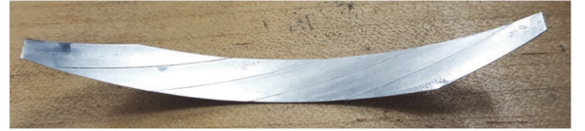
Fig. 4. Crossover laminate with 5 REBCO conductors soldered to copper foil.
