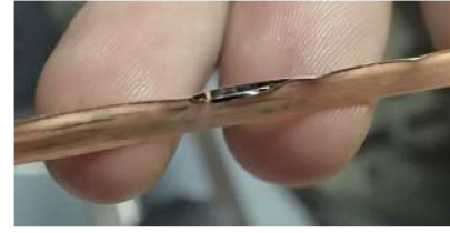
Fig. 11. A section of REBCO tape from the STNC coil showing high deformation and delamination along one edge.
