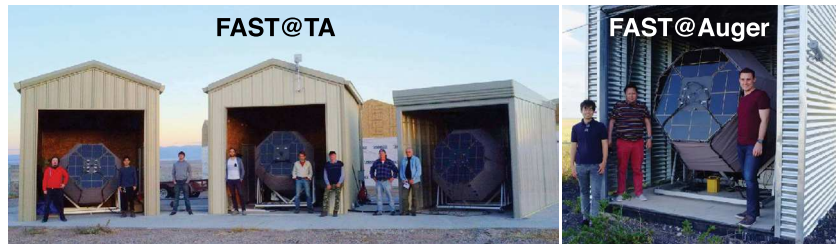
Fig. 59. The prototypes of the Fluorescence detector Array of Single-pixel Telescopes (FAST) installed at the Telescope Array Experiment and Pierre Auger Observatory, dubbed FAST@TA and FAST@Auger, respectively.
