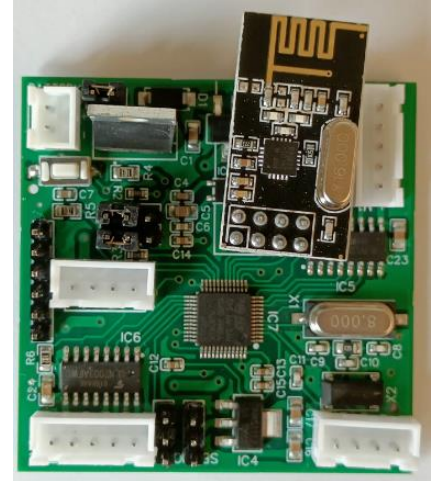
FIGURE 11: A PCB BOARD DESIGN WITH TRANSMITTER
