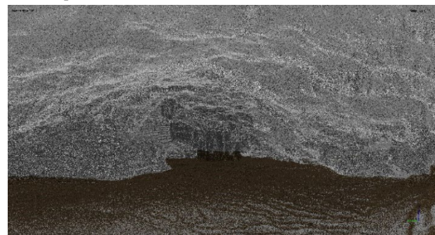
Figure 4. a) Aligning 2 overlapping scans in Register 360. b) Classified cave floor (brown) and unclassified cave wall and ceiling (grey).
