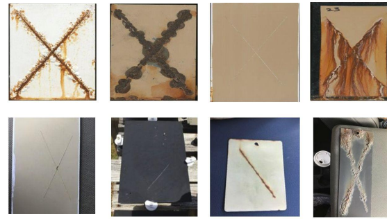
Figure 1: Corrosion test image panels. Top: Indoor laboratory environment tests. Bottom: Outdoor natural environment tests.
