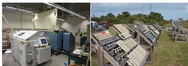
Figure 2: Indoor (left) and outdoor (right) corrosion testing environments.
