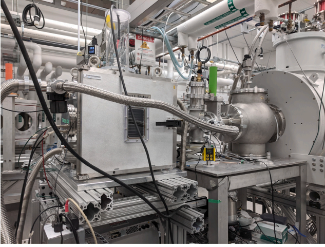
Fig. 2. Photograph of the ND-Cube attached to the TriSol beamline downstream of the third solenoid.
