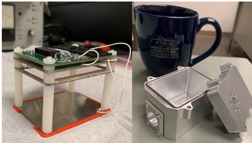
Fig. 1. Pictures of the internals of the ionization chamber (left) and detector body (right). The uneven wire spacing in the Frisch grid is an artifact of it being done manually and has since been improved.
