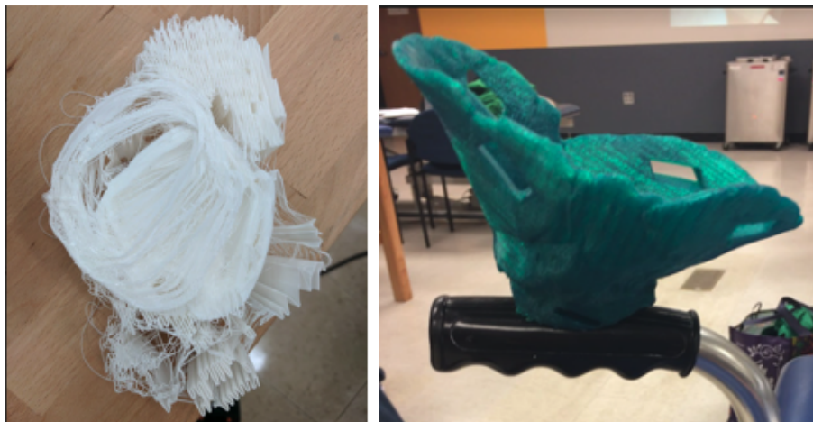
Figure 2: (Left) This image shows a failed cheetah print of an elbow bowl for case 2 in phase 1 and (Right) This image shows the successfully printed version of the image on the left.
