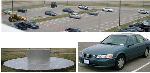
Figure 2: Optical images of parking lot being imaged in GOTCHA dataset, [18]. The scene contains a variety of calibration targets, such as primitive reflectors like the tophat shown, a Toyota Camry, forklift, and tractor.
