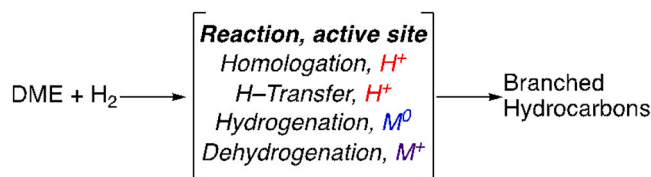
Fig. 1. Schematic of reaction pathways and corresponding active sites for DME homologation with co-fed \text{H}_2 over metal-modified BEA zeolite catalysts.
