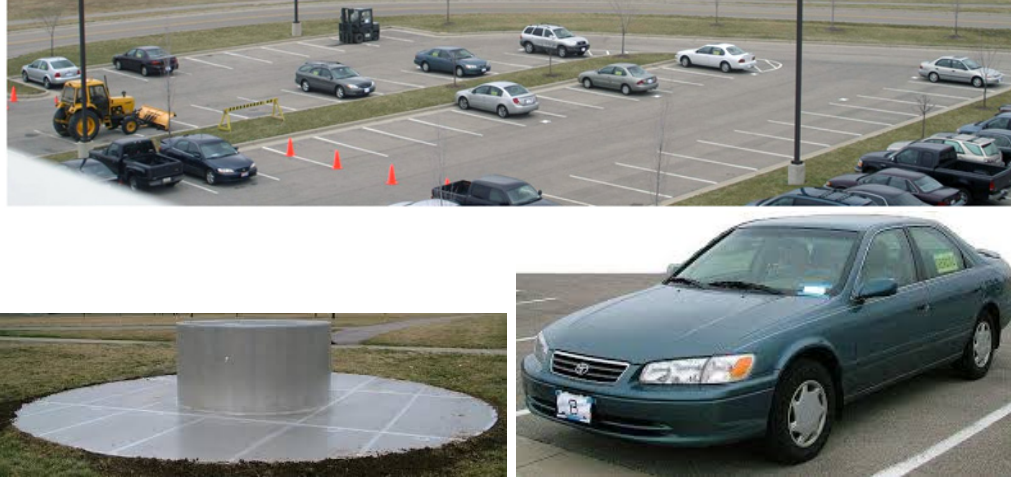
Figure 5: Optical images of parking lot being imaged in GOTCHA dataset, [13]. Note scene contains a variety of calibration targets, such as primitive reflectors like the tophat shown, a Toyota Camry, forklift, and tractor.
