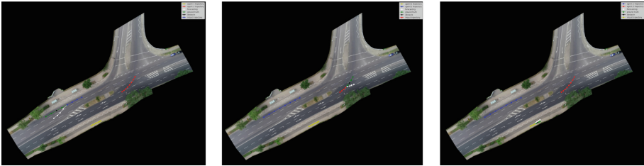
Fig. 4. Sudden obstacle visualization. In each image, the green trajectory is the ground truth and the white one is the predicted result. The black point is the sudden obstacle. The obstacle is placed in the ground truth trajectory. The white trajectory demonstrates that the agent successfully avoids the obstacle.
