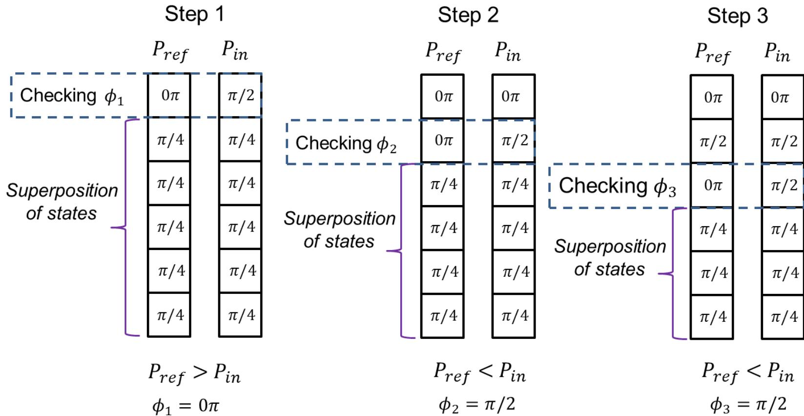
Illustration of the search procedure. There are shown the first three consecutive steps. At the first step all inputs from 2 to  $n$  are put into a superposition of states. There are two measurements to determine the “true” value of input 1. One measurement is  $0>$  + superposition the other is  $1>$  + superposition. The “true” input always provide the larger output power. It takes  $n$  steps with  $2n$  measurements to find the one of the  $2^n$  possible input combinations.
