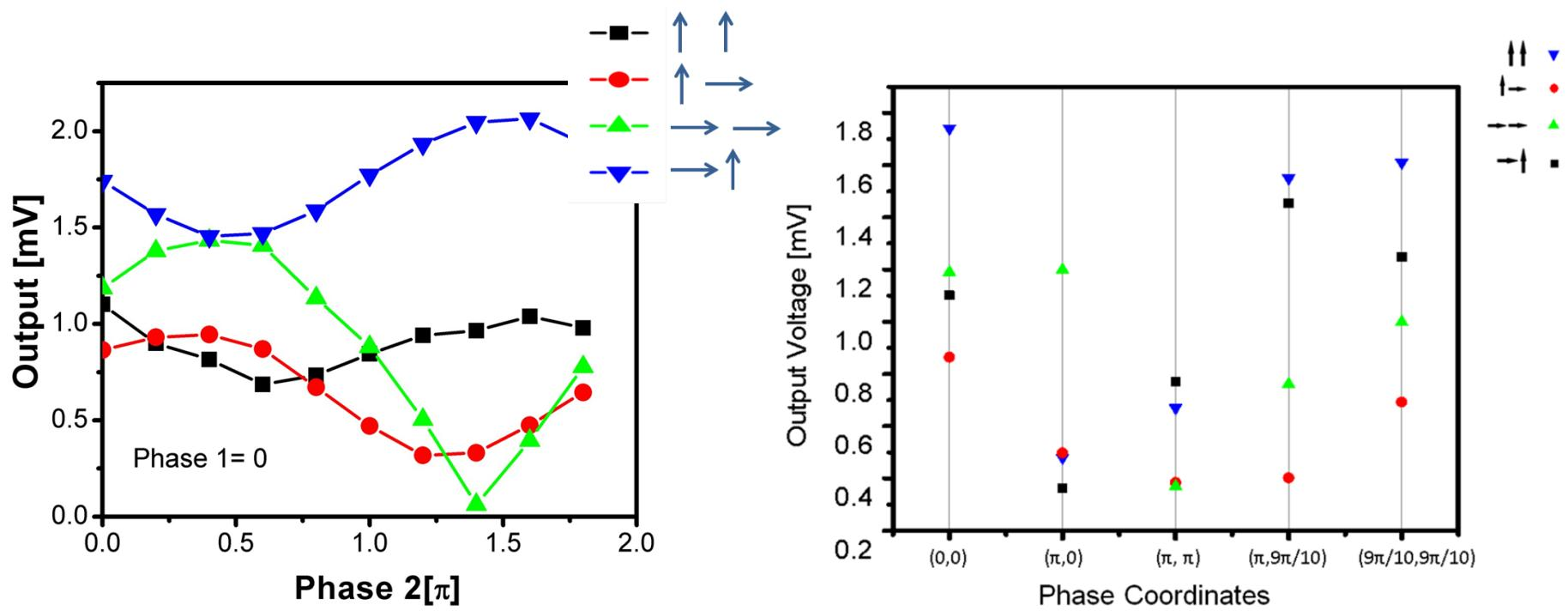
The graphs show the unique holographic signature of the magnetic structure with two magnets placed on the top of the junctions. The graph on the left shows the output in mV as a function of the spin wave phase 2 (the connection schematics are shown on the previous slide). The output oscillates with the phase difference as predicted by numerical simulations.
