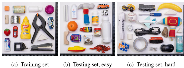
Fig. 9 Object sets used for training and testing. Both training and the test set easy include 15 objects while the test set hard has 20 objects. Objects were curated so that they were graspable by the Robotiq 2F-85 parallel jaw gripper from any configuration and visible to the Occipital Structure Sensor
