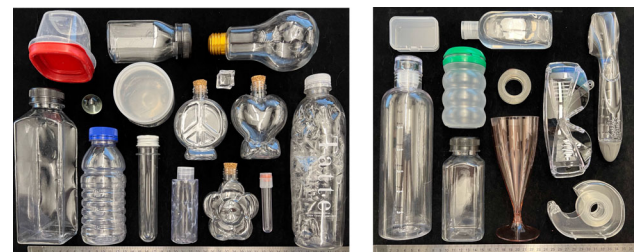
Fig. 10 Transparent object sets used for training and testing. The Training set includes 15 objects and the testing set includes 10 objects. Objects were curated so that they were graspable by the Robotiq 2F-85 parallel jaw gripper from any configuration
