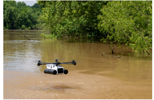
Fig. 8: The HexH2O hexacopter landing on water.
