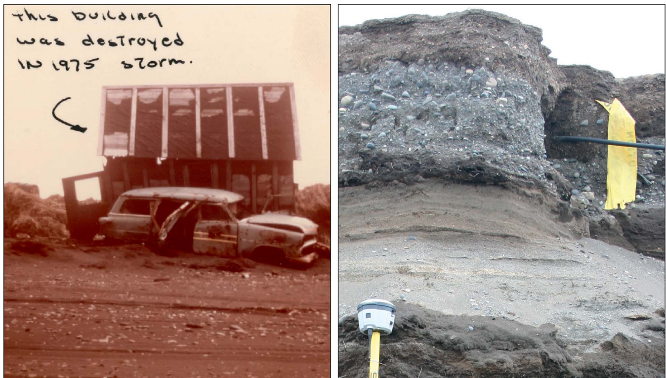
Figure 3. (Left) Photograph by Kvasager (1975) showing a structure and car destroyed by a 1975 storm. The beach is composed of glacially derived cobbles in sand. (Right) This picture of the eroded bluff underneath former Meshik shows the cobbles from the beach used for the road system. For scale, the GNSS antenna is 15 cm tall.
