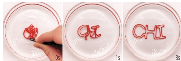
Figure 16: Shape recovery of the letter toy in a 60 °C water bath.
