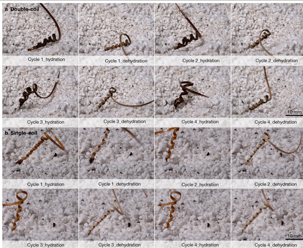
Extended Data Fig. 5 | Comparison of the self-drilling depth between a double-coiled and a single-coiled seed carrier. a–b, Photographs of four cycles of a double-coiled seed carrier ( a ) and a single-coiled seed carrier ( b ) at each hydration and dehydration state.
