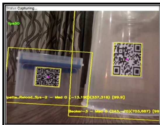
Fig 13: Multiple tools being detected with one in the background and overlapping bounding boxes.
