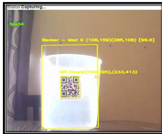
Fig 9: Detection from our custom model. Top left value represents the frames being processed per second.
