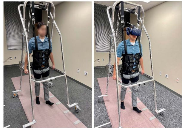
Figure 3: Participants were supported by a harness while they performed the timed walking task using the GAITRite system in real-world (left, face blurred) and virtual environment (right)
