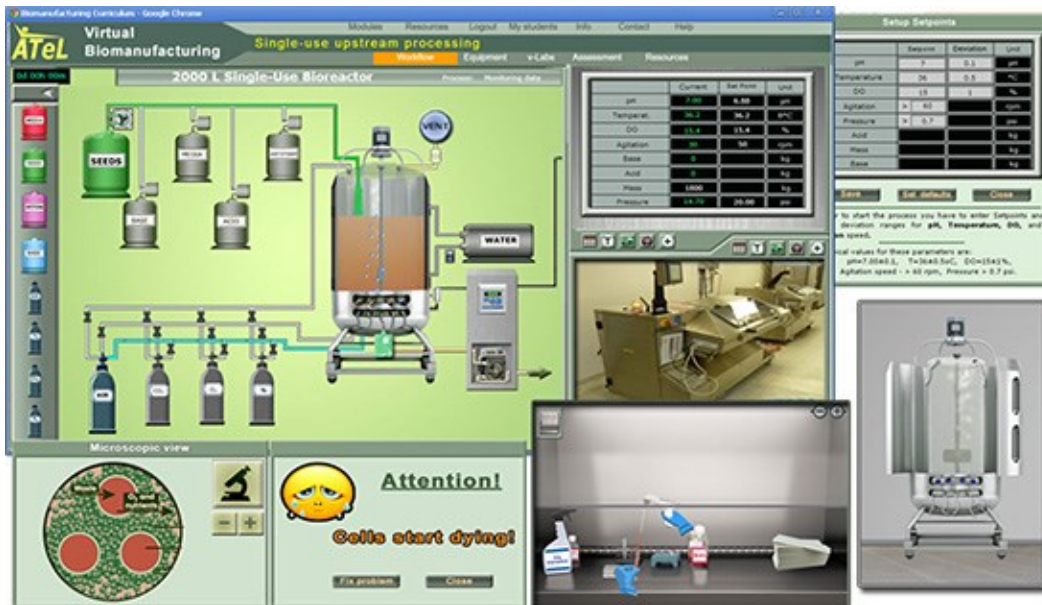
Figure 3. Screenshots of the Cell Growth lab, where a student can virtually assemble a disposable bioreactor and related production system and calculate an initial amount of buffer and cell culture. Then, he/she loads the system and controls the cell growth and performs the required procedures such as calibrating sensors, taking and analyzing probes, maintaining the appropriate temperature and atmosphere, etc. The system imitates abnormal situations involving the student in troubleshooting. The microscopic view visualizes the processes occurring in-side the bioreactor.
