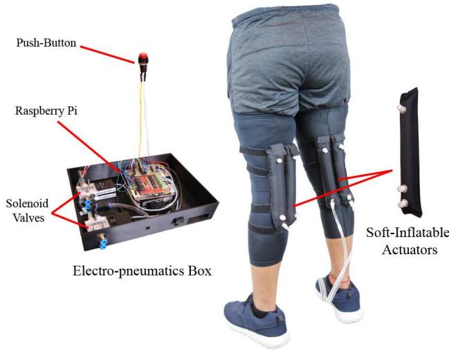
Fig. 1: The soft-inflatable exosuit system worn by a human subject. The system is composed of two soft-inflatable actuators for each leg, solenoid valves, Raspberry Pi and a push-button.
