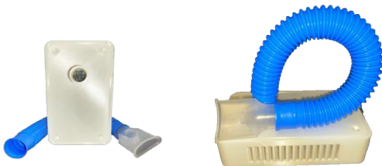
Fig.4. Physical Prototype of the spirometer (fully assembled)
