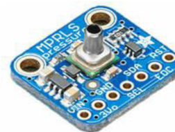
Fig.2. Adafruit MPRLS Pressure Sensor
