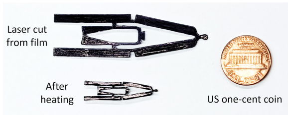
Fig. 14. A shrinking technique with polystyrene materials
