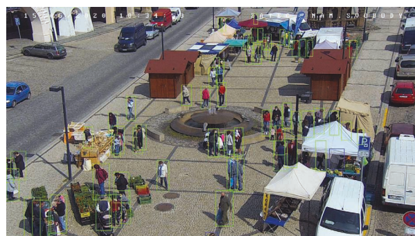
FIGURE 1. Three snapshots captured on different days from three locations. We counted the people in each image by hand and found 33, 85, and 70 people in each image, respectively. Pedestron found 31, 84, and 68 people, respectively. The right images show correctly detected bounding boxes containing people (green), false positives (red), and false negatives (blue). (a) Aydat, France, 11 August 2020. (Source: www.meteosurfcarnarias.com .) (b) Kerns, Switzerland, 29 December 2020. (Source: Snoweye.com .) (c) Žatec, Czech Republic, 15 May 2020. (Source: webcam.mesto-zatec.cz .)
