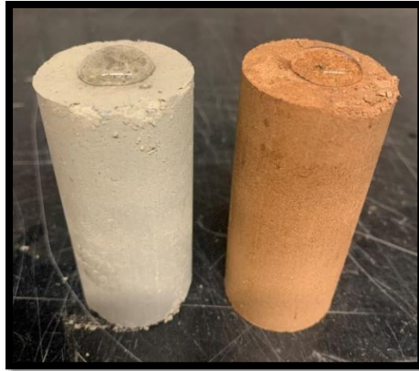
Figure 2. Water beading on surfaces of soil samples treated with chemical agents (diameter of samples are each 32.85 mm)
