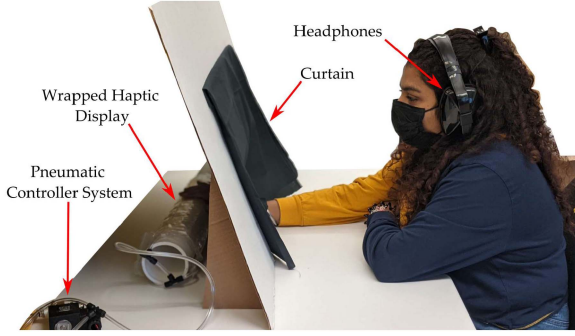
Fig. 3. Experimental Setup. The participants were instructed to sit at the desk right in front of the curtain and put on hearing protection headphones.
