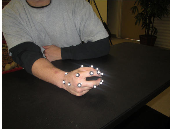
Fig. 6. Optical motion capture of a subject performing grasping of a small pen using their thumb, index and middle fingers.
