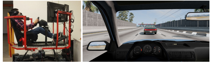
Fig. 3. Real-time 3D simulation with motion feedback.
