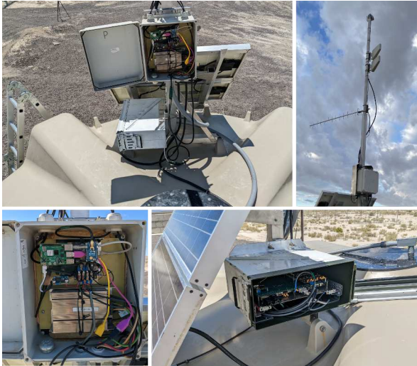
Figure 4: Auger@TA station components deployed in the field. Top left: Positioning of the E-kit and the NEMA box on the communications mast. The TPCB and a Raspberry Pi for the communications system can be seen. Top right: Communications mast with GPS (top), 4G (middle), and YAGI (bottom) antennas in place. Bottom left: Close-up of the NEMA enclosure. Bottom right: Inside view of the E-kit box with the UB on the drawer slides.
