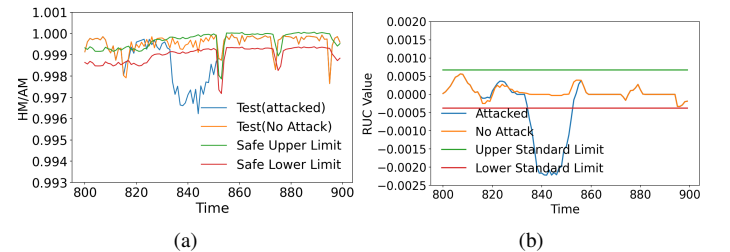
Fig. 12: Alternating Switching Attack with \delta_{avg} = 0.5 amps (a) Ratio Snapshot; (b) RUC(T) Snapshot.
