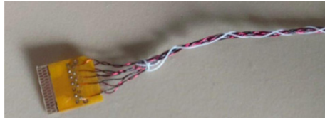
Figure 2. One end of an electrical link (e-link) bundle that has five twisted pair channels: one channel for a control link and four channels for data readout.
