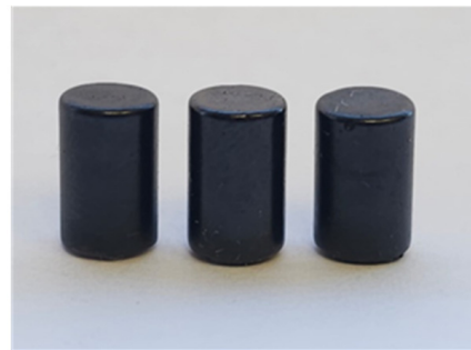
Figure 1. Shaping of SunBG 90 by pouring a molten sample into silicone mold (a) to produce tiles (b). A similar process can be used to produce a variety of other shapes such as the cylinders that were used for compressive testing (c).
