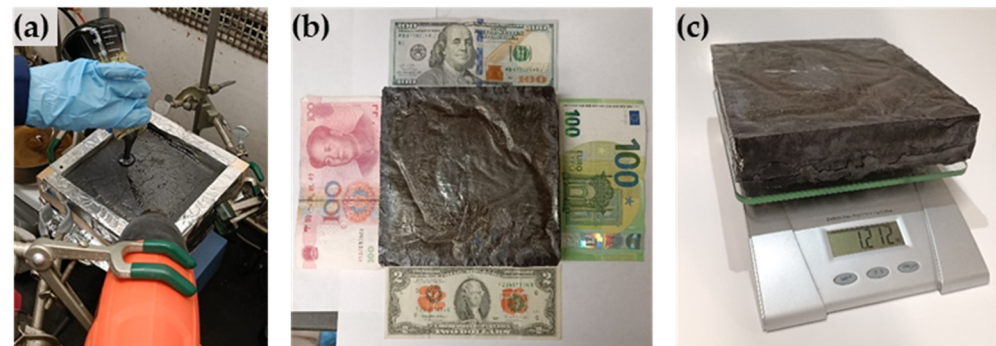
Figure 2. Pouring molten SunBG 90 into a foil-lined brick mold (a) to form the brick (b) used for ISO 8302, with a mass of 1.212 kg (c).
