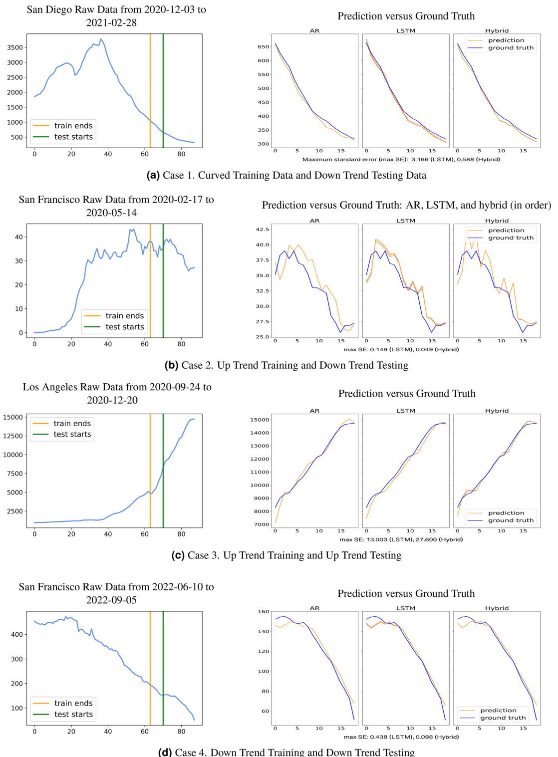
Figure 3. The left panels show the training and testing data. The right panels show the ground truth versus forecasts of the AR, LSTM, and hybrid model, respectively. We display the average prediction (solid line) with 2 times standard error (shaded region). The standard error across 100 runs are reported for LSTM and hybrid. The hybrid model is more stable than the LSTM.
