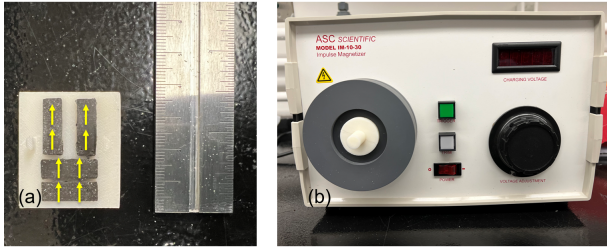
FIGURE 10: Ferromagnetic beam magnetization. (a) The beam is placed in the 3d printed holder, with yellow indicating the residual magnetic flux density of four beams after the magnetization process. (b) The model IM-10-30 Impulse Magnetizer used for the magnetization process.
