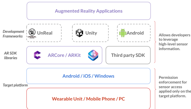
Figure 2: AR application developers use different frameworks and libraries that provide high-level functional APIs to access sensor information. These frameworks, however, do not provide any permission enforcement and default to the target platform access control.
