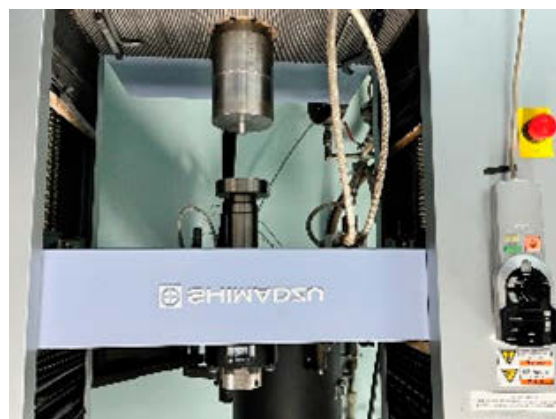
Figure 7. Floor testing machine Autograph AG-X 100 kN, Shimadzu GmbH.
