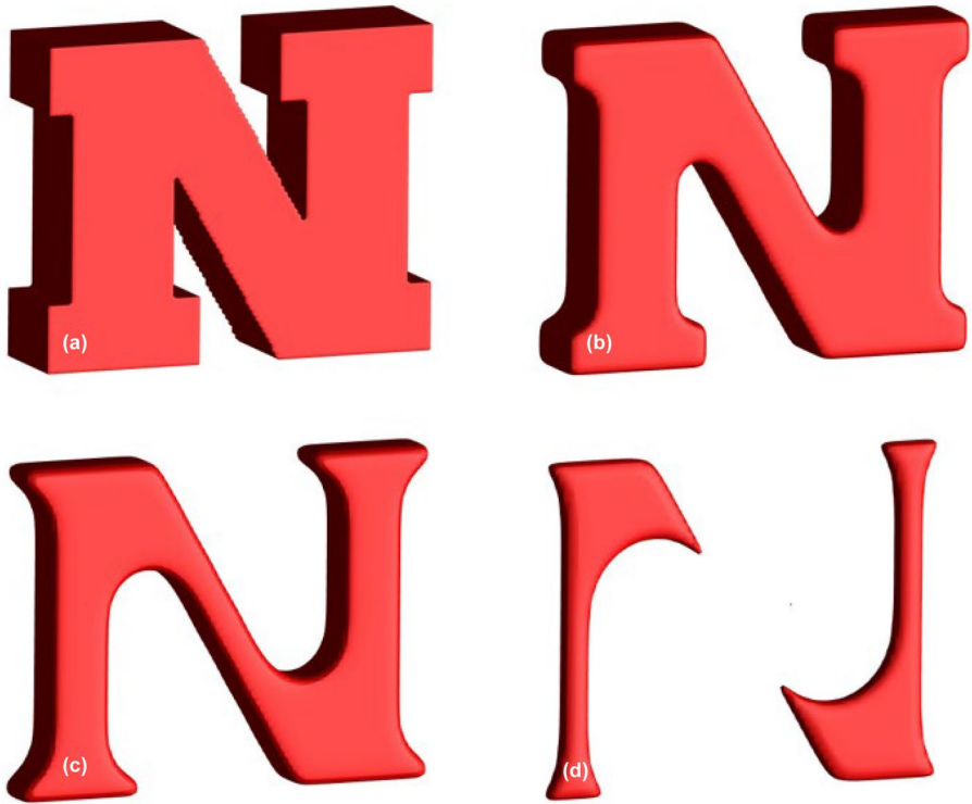
Fig. 6 Uniform corrosion of a complex shape at a 0 s, b 100 s, c 200 s, and d 300s
