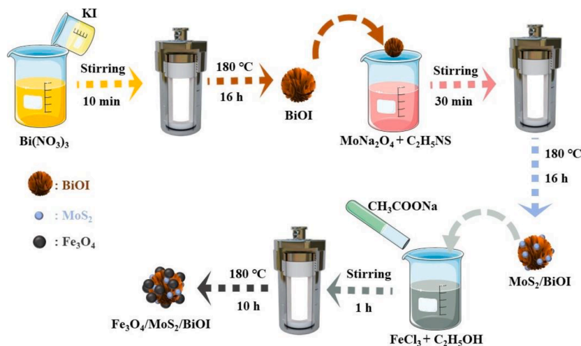
Fig. 1. Process flow diagram for synthesizing photocatalyst.
